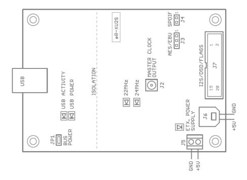
Figure 6-1 – Connectors, LED's and jumpers location
