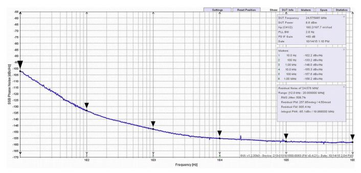
Figure 3-1 - Master Clock generator phase noise plot
