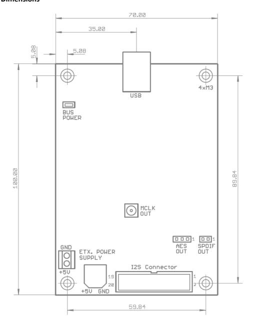
Figure 6-3 – Mechanical dimensions in millimeters
