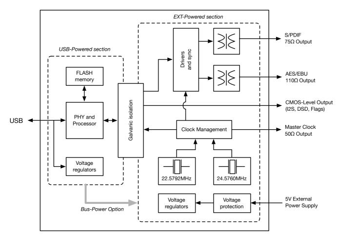
Figure 1-1 – XU2S Functional block diagram
