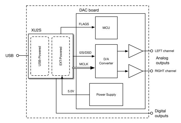
Figure 5-1 - eR-XU2S integration with a DAC board
